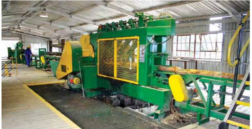
*The chipper saw at Glenhorpe Mill, used to cut logs on both sides.*
