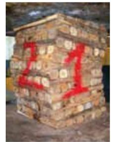
Pencil prop before and after testing. Total load is around 30 tons with a yielding of 250 mm. Initial length is 2.4m.
