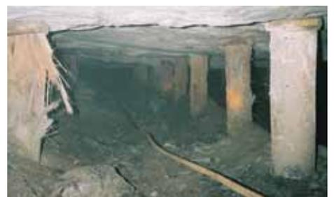
*Top: Loading product at Glenhorpe Mill. Above: Pencil props doing the job they were designed for underground.*
